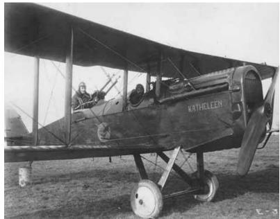
best model. A relocated fuel tank, a change in the landing gear, and one piece plywood body sections were incorporated. Only 13 of these improved aircraft were made before the war ended and production was halted.
