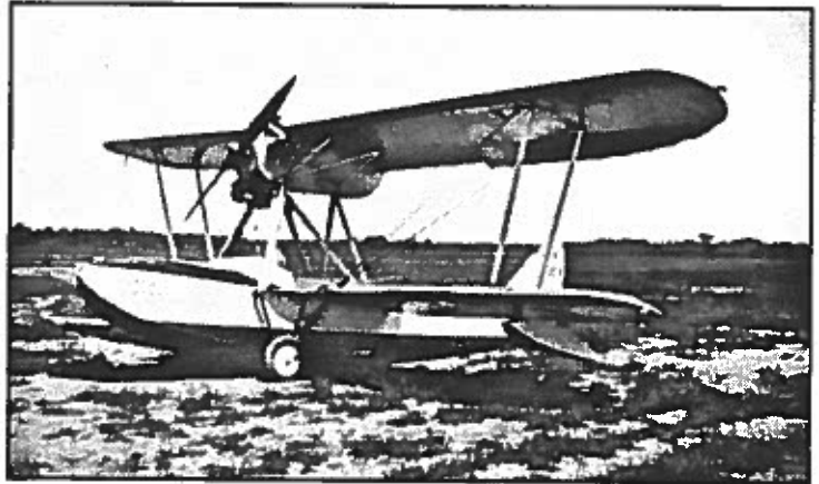
Savoia-Marchetti S-56 Amphibian NC-380-N with 100 hp Kinner K-5 engine.
